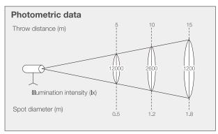
\* The above spot diameter is minimum data. The maximum spot diameter is 1.5 times compared with minimum data.
