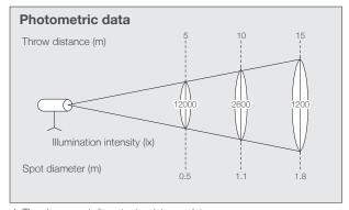
\* The above spot diameter is minimum data. The maximum spot diameter is 2.3 times compared with minimum data.
